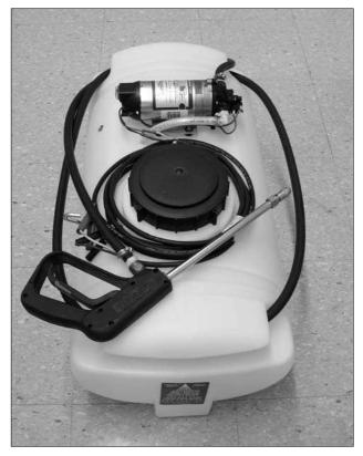
Hand sprayers are less cumbersome for applying liquid herbicide to small or targeted areas.
