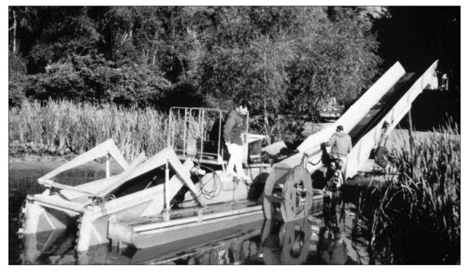
Cutter harvesters such as this one can cut and haul up to 15 tons of plant material at one time. Smaller units can be fitted onto boats for use in water bodies of more limited size.
