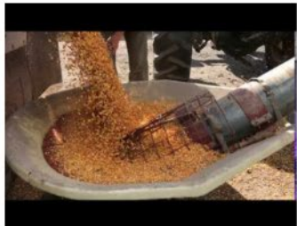
Transferring Corn From Truck To Bin Using An Auger
