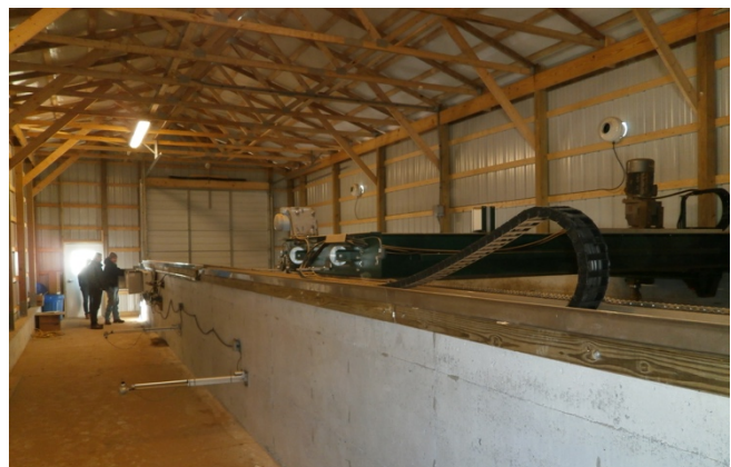
Figure 1. Green Mountain Technology's composting system at Glamour View Farm is housed within a permanent structure. Figure 2. The Earth Flow composting system features automated mixing and aeration equipment. Photo credits: David Kann.
